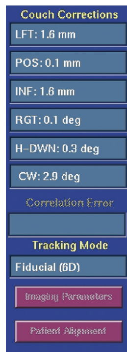
Fig. 5. Couch correction values. Couch movement is not performed if its values are within the tolerance limits.
