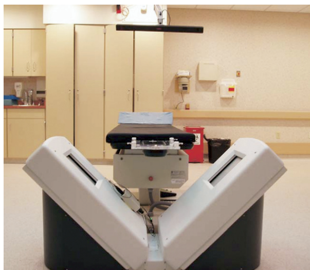
Fig. 4. An x-ray detection system consisting of 2 flat panel detectors mounted both sides of the treatment couch.
