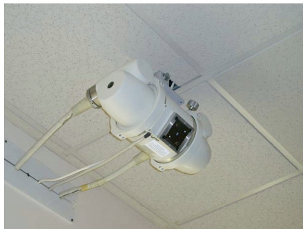
Fig. 3. A kilovoltage x-ray source mounted on the ceiling to produce orthogonal live radiographs.
