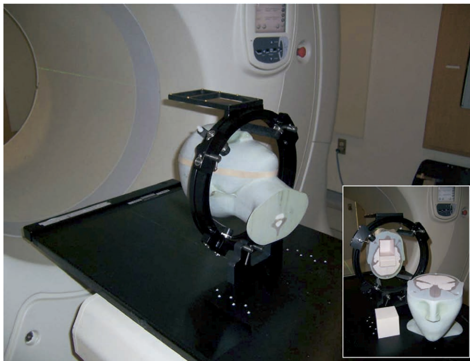
Fig. 8. SRS head phantom setup for testing localization accuracy of dose to a small target. Inset photo shows the internal film dosimetry block.
