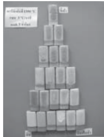
Figure 8. Glaze fired under condition #6; maximum temperature 1,350°C; heating rate 5°C/min; soaking time 3 h under reduction
