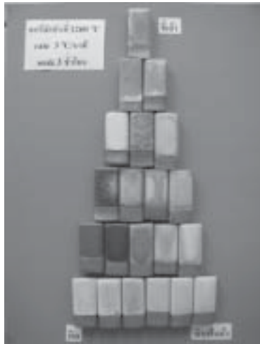
Figure 7. Glaze fired under condition #5; maximum temperature 1,260°C; heating rate 3°C/min; soaking time 3 h under reduction
