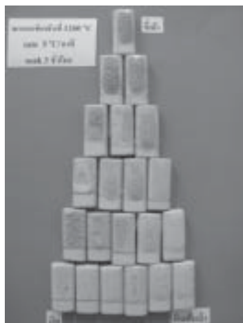
Figure 4. Glaze fired under condition #2; maximum temperature 1,260°C; heating rate 5°C/min; soaking time 3 h under oxidation
