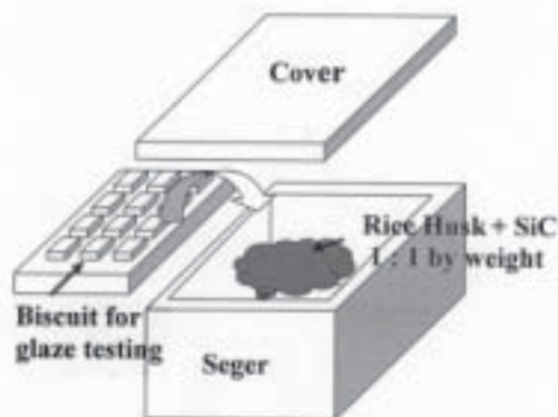
Figure 2. Crucible setting for reducing firing condition
