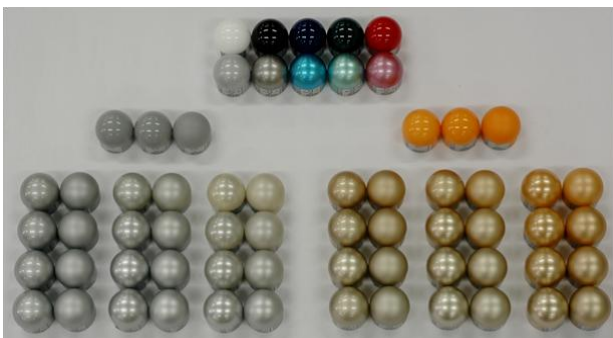
Figure 2. Metallic painted hemisphere samples differing in their composition of microstructure.
