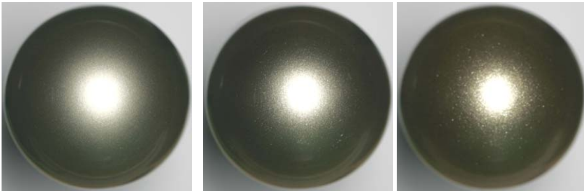
Figure 3.5: Effect of flake size variation on the appearance of a gold coated surface. From left: coated surface with average flake size 15, 20, 25 micron respectively in their microstructure. All the samples have same flake density of 8%.
