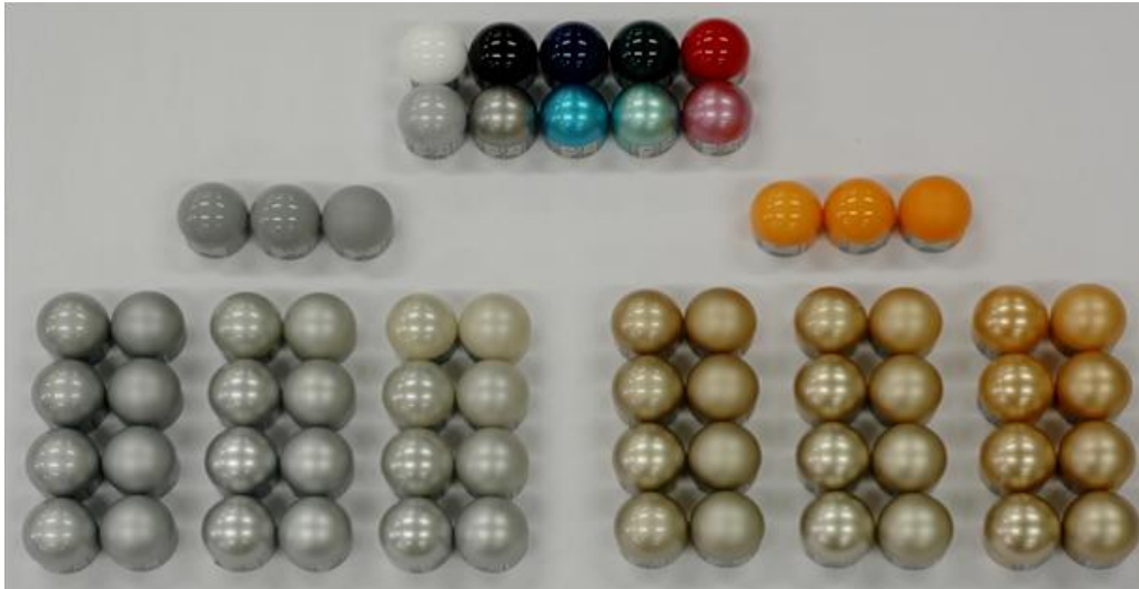
Figure 4.2: Coated samples differing in their microstructural composition
