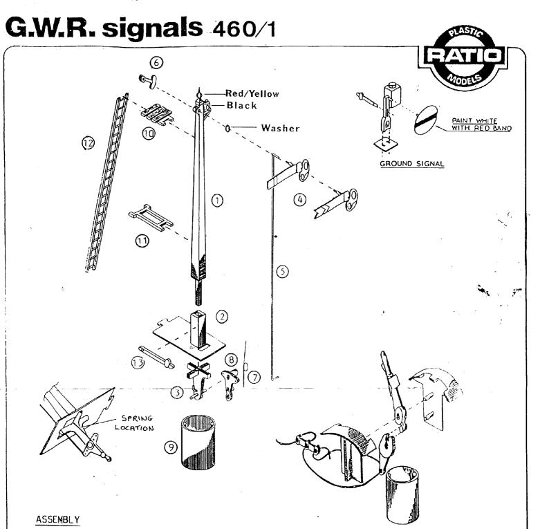
Remove approx 1/8th" from post location spigót. Glue post (1) into base (2). When dry, cement quadrant (3) under base. NOTE. This must be fitted the correct way around (see drawing) and stand at 90° to base.
