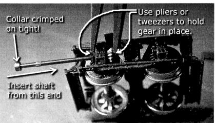
24. The toughest part is getting the shaft into and through the first gear. Once you've finally accomplished that, use your pliers as shown to apply pressure to the back of the gear, pushing the shaft onto your work surface to persuade it through. Do not push on any part of the truck to help accomplish this task. Push *only* on the shaft itself or on the gear.
