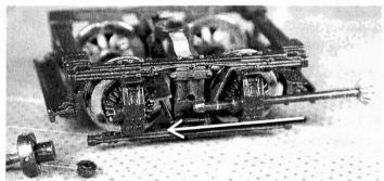
Engage gear \_\_\_\_\_ with wheel gear Push shaft through gear and journal box. Stop at knurl.
