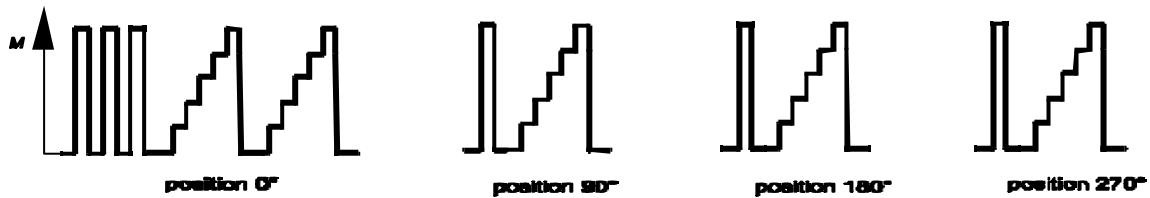
Fig. D.3: Example of preloadings and sequences for torque measuring devices with square drive, a minimum 5 steps, only increasing series and 0,1\% \leq U < 1\%
