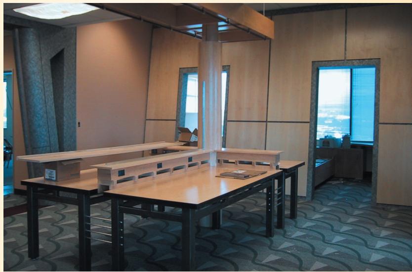
Figure A. Offices of the Institute for Creative Technologies. Tilted wall paneling forces sound upward and downward, providing privacy without the constriction of a cube environment. Open work areas facilitate collaboration while small offices that can be closed off with curtains provide privacy and bunk beds for rest during extended working hours.
