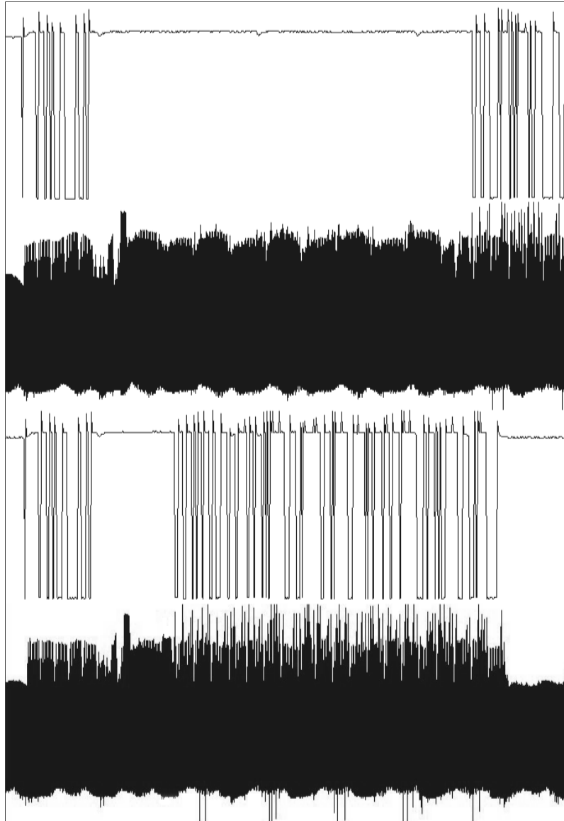
The acquisitions from top to bottom: The I/O trace of a normal AES execution and its power consumption, where the rounds can be seen. This is followed by the I/O trace of an AES execution where the number of rounds have been reduced to one and the power consumption shows the reduction in the number of rounds.
