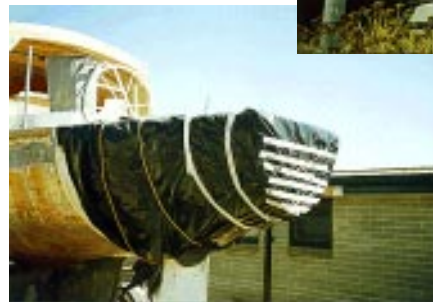
Top: Ready to plaster, note the tennis ball steering limiter buffers. Above: 6mm steel rods welded to original steel, new transom 16mm rebar. Left: Plastered and curing for 1 month with siphon dripper and sprinkler inside hull turned on a couple of times a day.
