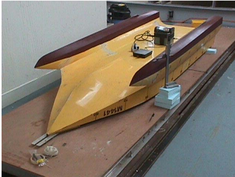
Figure A.6. Photograph of the levelled model and the marking method of the draught lines.
