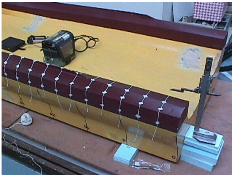
Figure A.7. The method of marking equally spaced stations with cords and measuring vertical and transverse co-ordinates of points with the height gauge and caliper.
