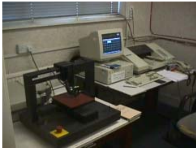
Figure 6.5. Photograph of the optical measurement system, used to analyse the sample coated plates.
