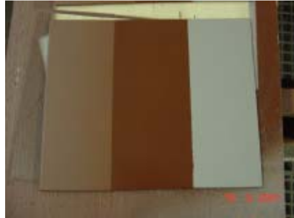
Figure 6.16. Composition of the CSPC scheme: (from right to left): primer, primer + 1 coat of SPC, primer + 2 coats of SPC = final scheme
