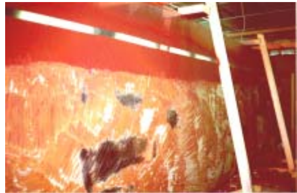
Figure 3.25. Patches of exposed aluminium after removal of the Tin-free SPC.
