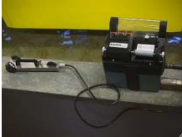
Figure 2.14. The BMT (ex-BSRA) Hull Roughness Analyser, which was used for measuring the roughness of the surfaces tested in the experiments of Chapters 3 and 5.
