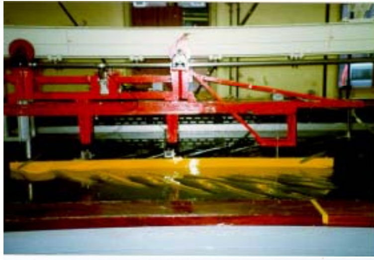
Figure 3.12. The flat plane coated with the Foul Release towed at speed of 1.373m/s
