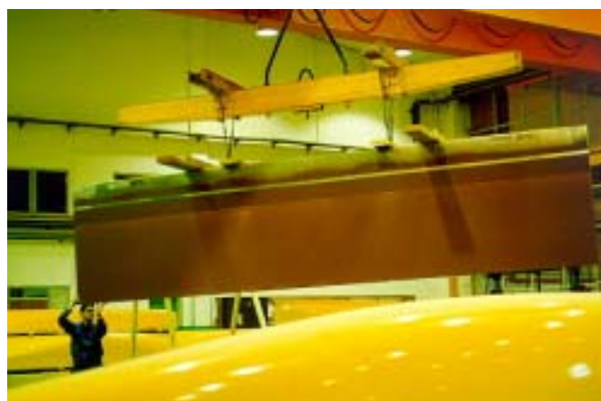
Figure 3.23. The appearance of the SPC surface after testing: the different colour shade due to polishing of the coating under the waterline is clearly visible.
