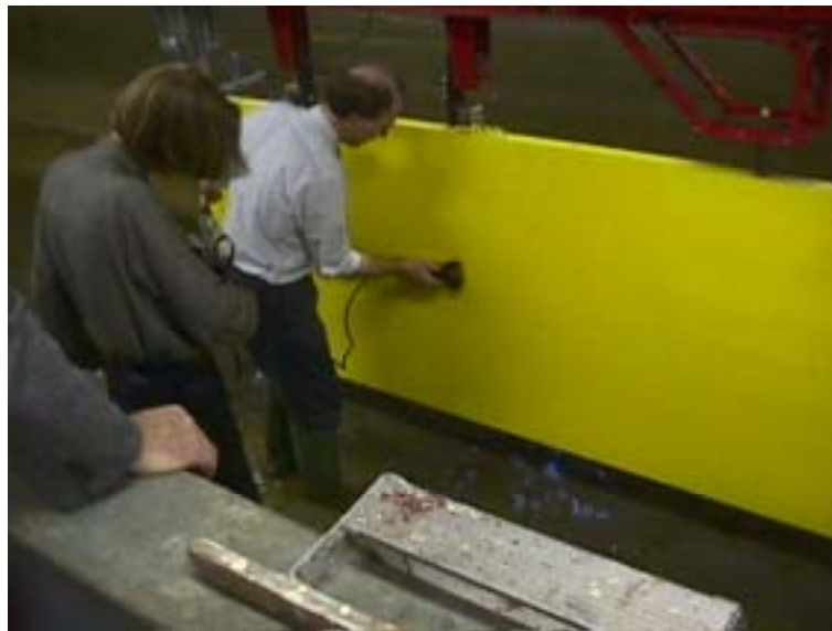
Figure 3.7. Measuring the Foul Release roughness of the suspended plate.
