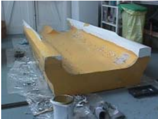
Figure 3.47. Stripping of the Foul Release coating.
