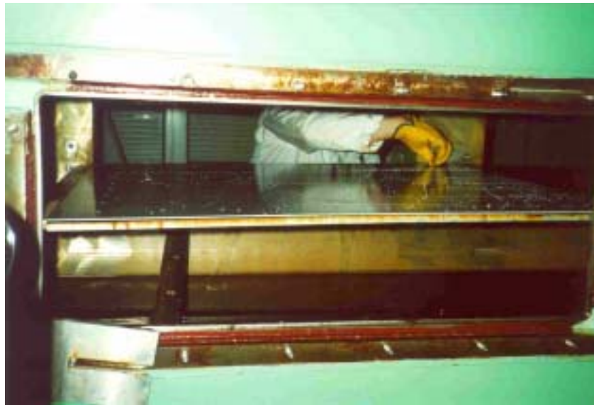
Figure 5.45. The CFR test plate is being mounted on the supporting plate by countersunk screws.
