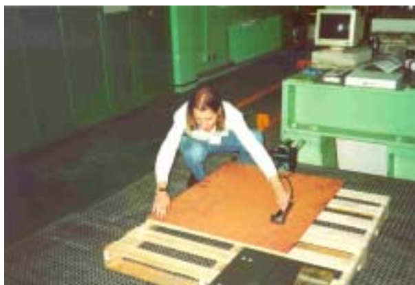
Figure 5.56. Roughness measurement with the BMT Hull Roughness Analyser after testing
