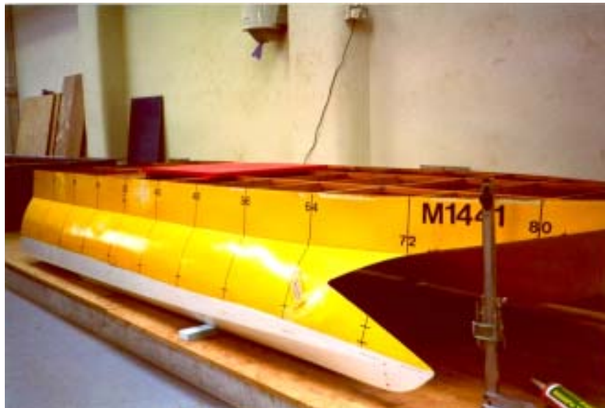
Figure 3.44. Photograph of the model, positioned to level trim. The waterline is marked in green on the coated surface and the studs are put in 135mm aft of the bow.
