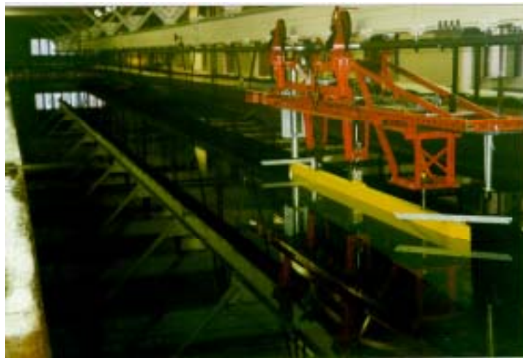
Figure 3.11. The flat plane coated with the Foul Release fitted to the towing carriage.
