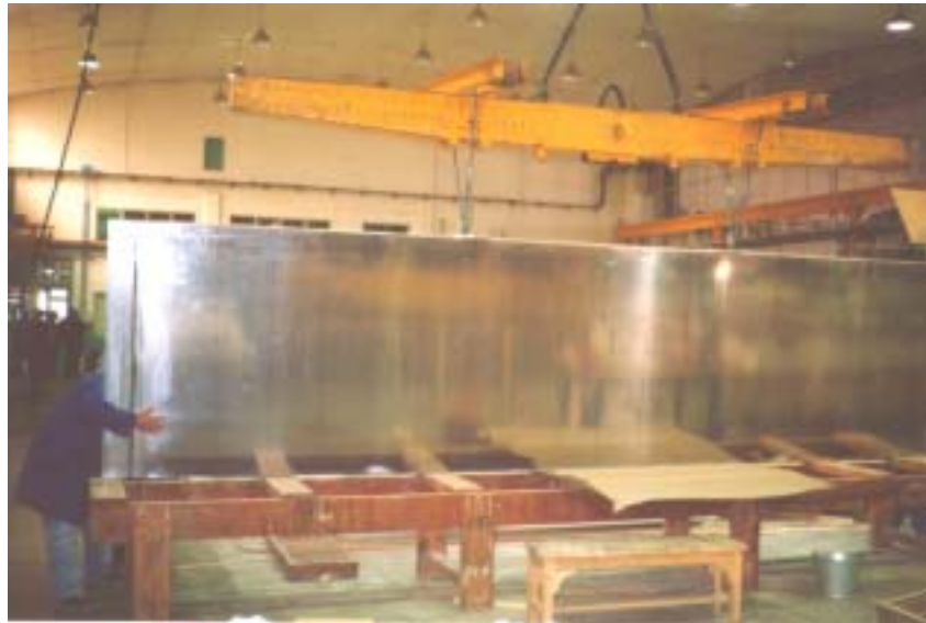
Figure 3.19. The flat plate, marked with vertical and waterlines, prior to first immersion.
