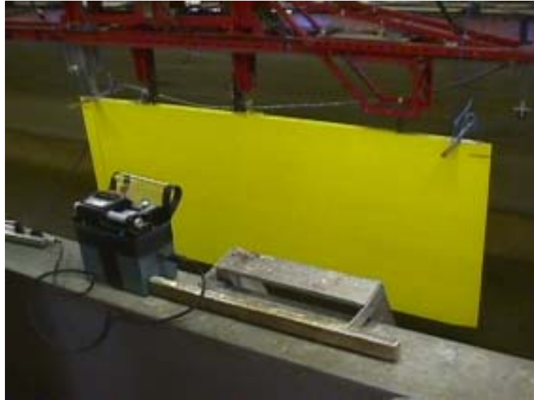
Figure 3.2. 2.55m long flat plate (coated with the Foul Release) suspended from the towing carriage
