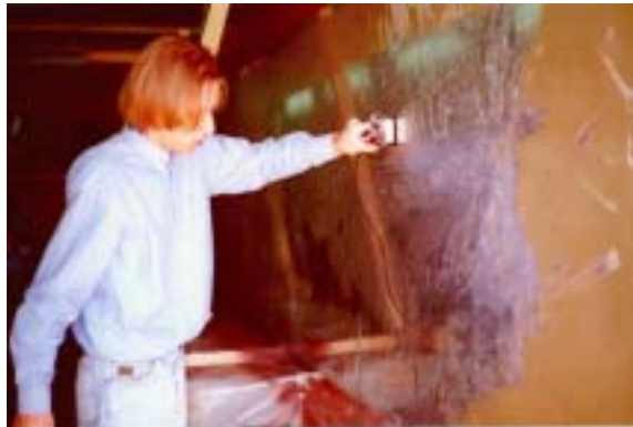
Figure 3.35. Measuring the roughness of the scraped surface
