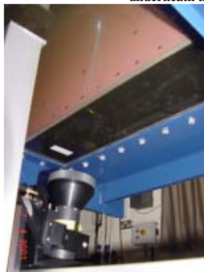
Figure 5.8. The LDV Set-up: traverse positioned underneath the tunnel
