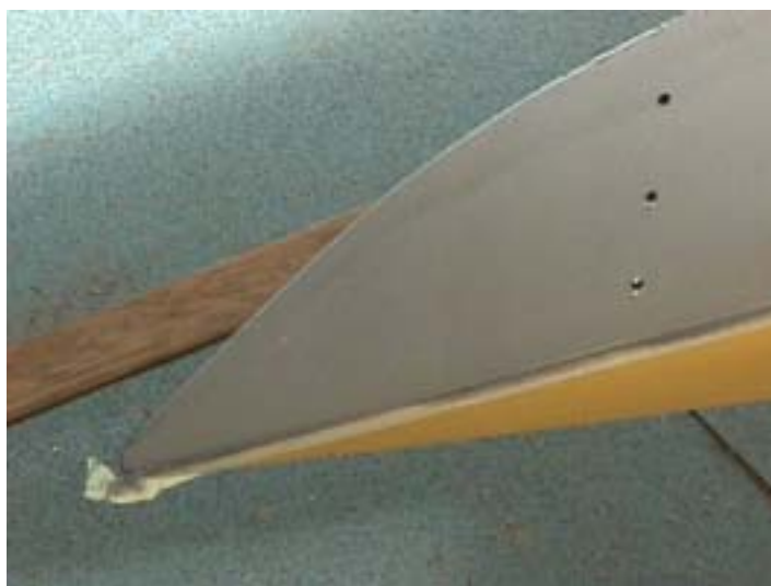
Figure 3.59. Paint thickness build-up of the Foul Release system around areas of high curvature.
