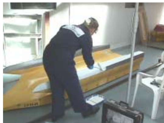
Figure 3.46. Application of the topcoat
