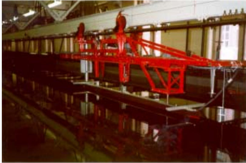
Figure 3.10. The flat plane coated with the Tin-free SPC fitted to the towing carriage.
