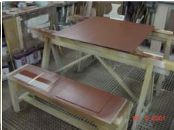
Figure 5.51. Final look of the CSPC scheme with sample plates front left showing the build-up of the SPC scheme
