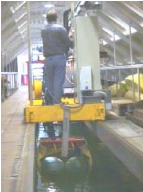
Figure 3.42. Photograph of the model attached to the carriage.
