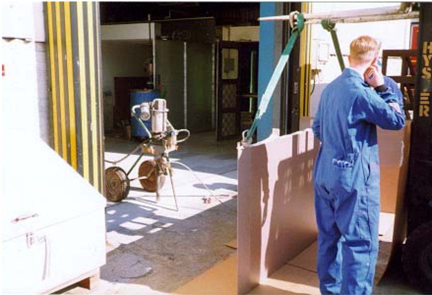
Figure 3.4. Outdoor application of the second and final coat of Tin-free SPC (July 9, 1998).
