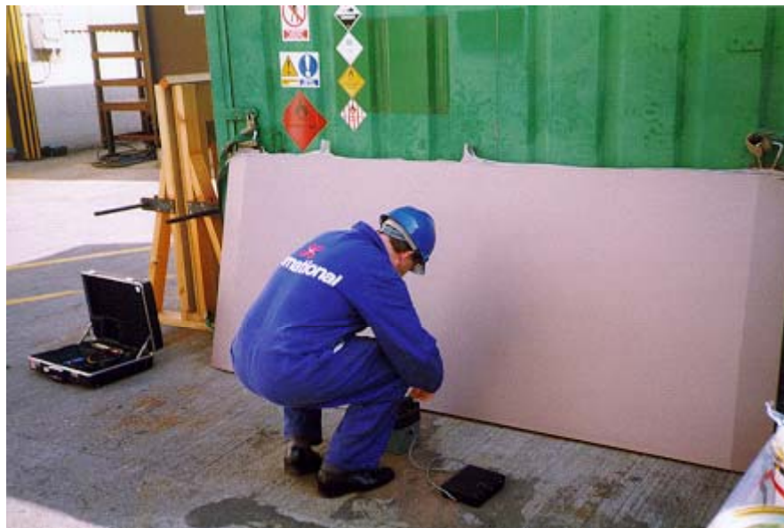
Figure 3.5. Measuring the roughness of the Tin-free SPC surface with the BMT Hull Roughness Analyser.
