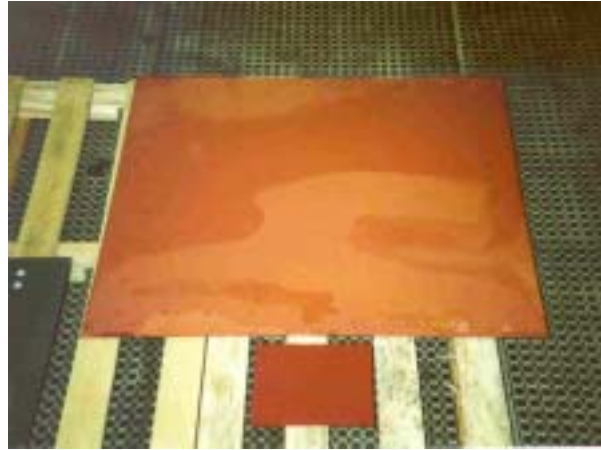
Figure 5.52. CSPC test specimen after testing. Sample plate was not immersed.
