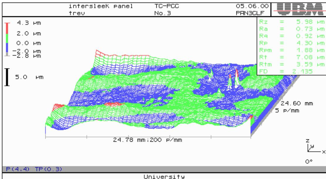
Fig. 2. Laser profilogram of a sample aluminium plate coated with a foul-release scheme
