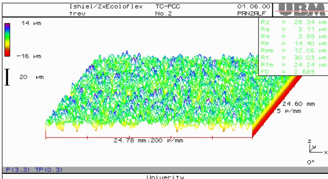
Fig. 3. Laser profilogram of a sample aluminium plate coated with a TBT-free SPC scheme
