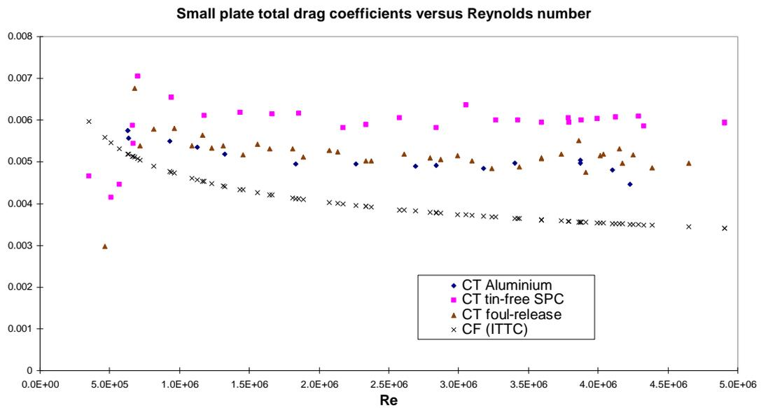
Fig. 5. Total resistance coefficients against Reynolds number of the three tested surfaces in the Newcastle towing tank
