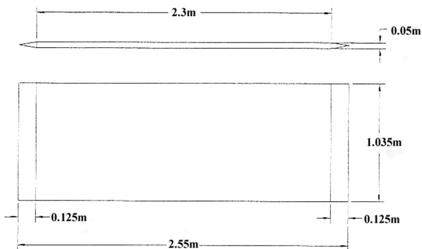
Fig. 4. Dimensions of the plate used in the Newcastle towing experiments
