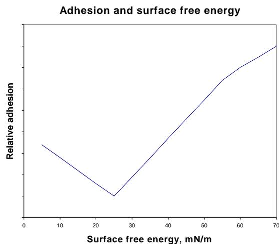
**Fig. 1** The relationship between surface free energy and adhesion<sup>after 2</sup>
