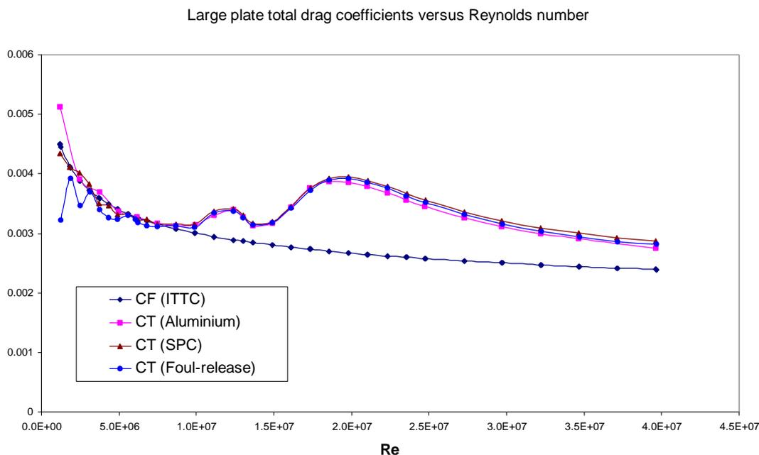
Fig. 8. Total resistance coefficients against Reynolds number of the three tested surfaces in the CEHIPAR Calm Water Tank
