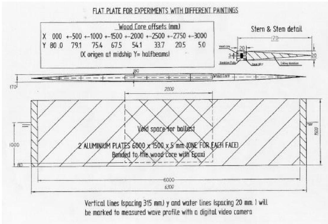
Fig. 7. Particulars of the plate used in the CEHIPAR towing experiments
