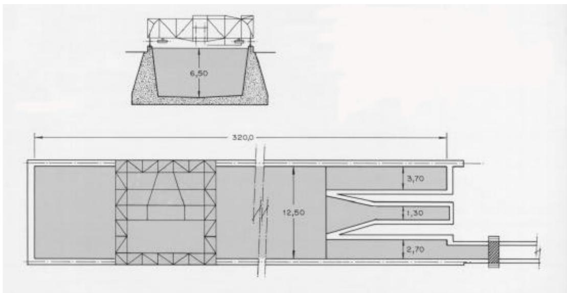
Fig. 6. Dimensions of the CEHIPAR Calm Water Tank
