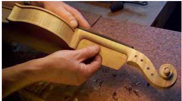
Derek uses callipers and a template to check the shape of the neck.
