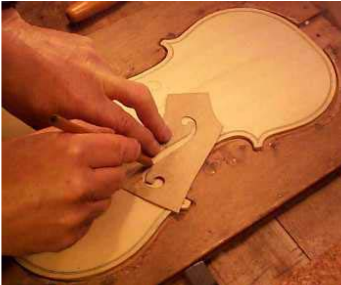
The template is placed on the front plate and drawn round with a pencil.
