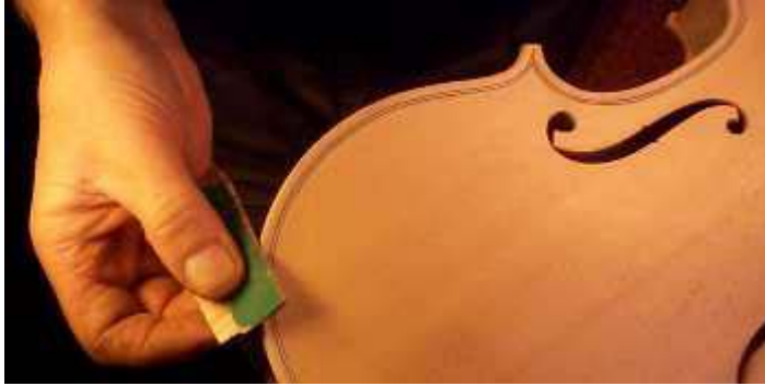
Above, a cork is used to support the abrasive paper as Derek shapes the corner. Left, a thin strip of wood is used as he shapes the bottom bout.
