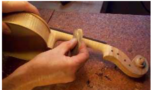
Finally Derek finishes the neck off with a scraper and with abrasive paper.
