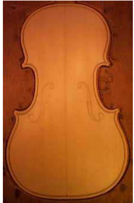
The template is placed on the front plate and drawn round with a pencil.
