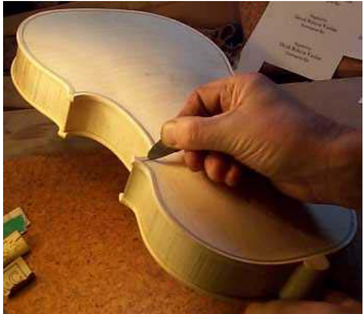
Here Derek uses a small teardrop shaped scraper around the margin of the instrument, where the arch rises up to meet the edge.
