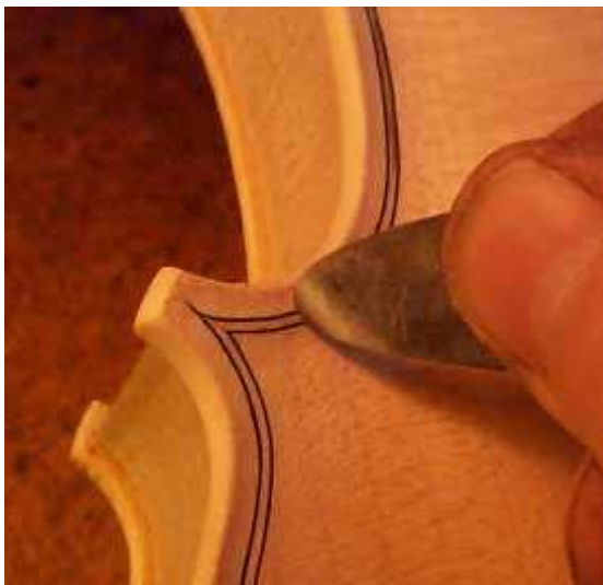
This picture shows how the edgework and the fluting over the purfling blend together.
