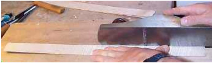
The rib is placed on a shooting board and planed to the right depth for this stage.
