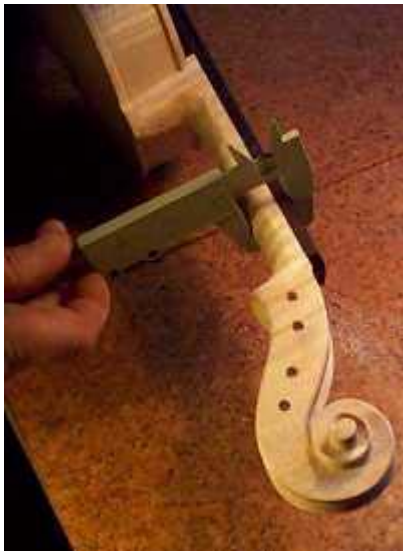
Derek uses callipers and a template to check the shape of the neck.
