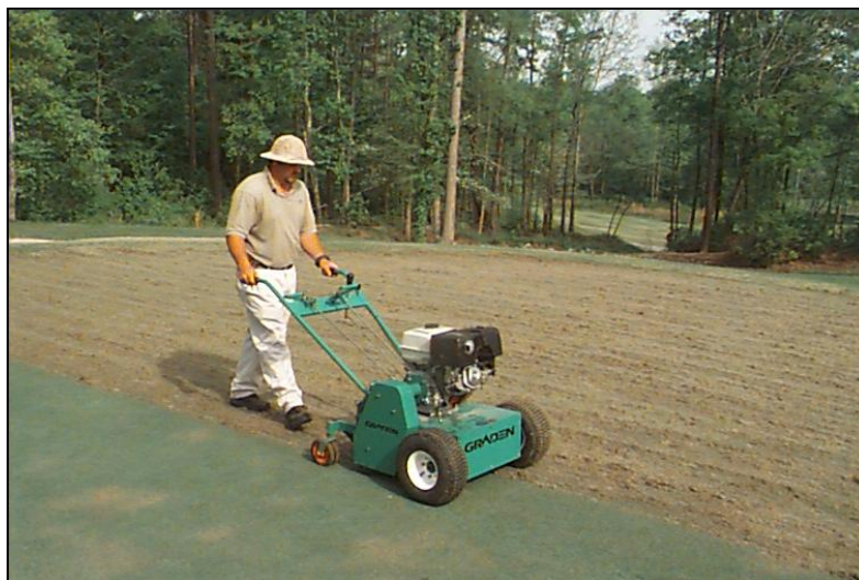
The Graden vertical mower has been used successfully by a number of courses to remove excess organic matter in the surface of greens and help with the incorporation of sand topdressing.
