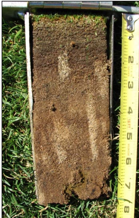
No. 5 profile shows nearly 3-in. of thatch and organic matter directly above soil that does not appear to fall within USGA specifications. Note the light-colored sand channels where aerification holes have been filled with quality topdressing sand.
