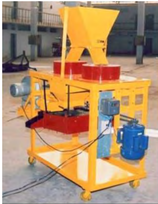
CIPHET developed castor pod decorticator
