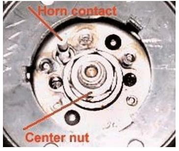
Remove the safety clip from the steering shaft, then remove the nut. You might have to have an assistant help hold the wheel while you turn the nut loose. Install the bolts from your steering wheel puller into the tapped holes in the wheel, and turn the puller screw to release the wheel from the steering shaft.
