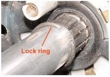
right side of the column holds the lock cylinder in place. Before removing the lock cylinder, make sure to hold the plastic/metal foil contact assembly in place so it's not lost down the column when the lock is removed. This switch assembly is actuates the key warning buzzer/chime.
