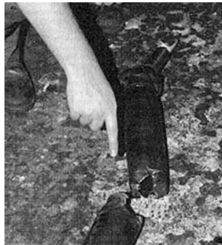
Inland Driveline's Jeff Gilroy offers the results of driveshaft failure due to operation at critical speed.
