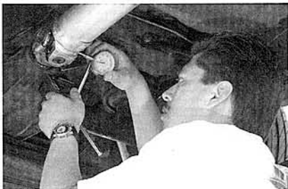
Powertrain Industries' Brian Arvizo measures pinion yoke runout. Mount the dial indicator securely. You must index as close to the center of each U-joint cap as possible and make sure the plane of the U-joint cap is 90 degrees to the dial indicator pintle when the reading is taken.
