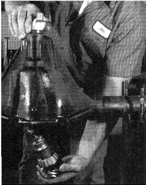
Many rear axle service shops recommend Timkin roller bearings, and that's what Jim Cook installed in our Malibu's 12-bolt, along with the new pinion yoke.
