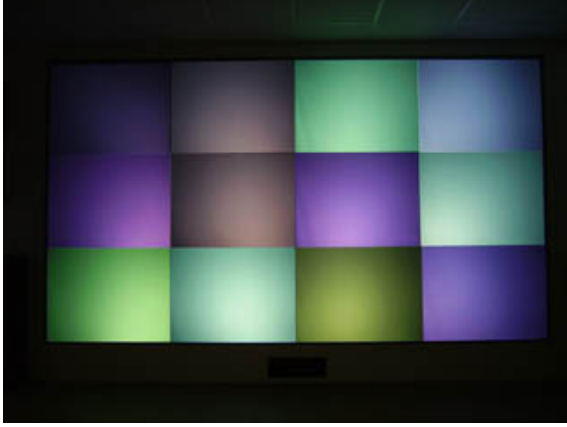
Figure 2: Uncalibrated Multi-Projection Wall
