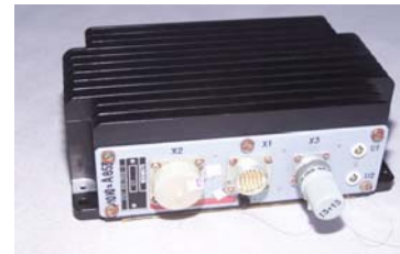
Power Converter Figure 14
