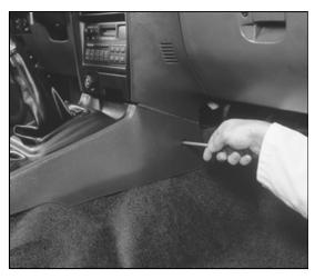
4. Remove the dust cover plate by removing five nuts and one bolt. Proceed to slide the boot of the dust cover over the handle of the shift change lever (and over the transfer lever on the 4X4).
