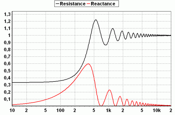
Figure 7: Finite exponential horn terminated by an infinite pipe.
