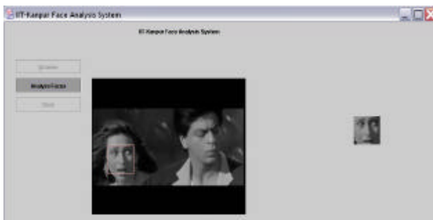
Figure 6. The Relevant face being tracked in subsequent frame. Note that, introduction of a new face has no significance on the efficiency of the system.
