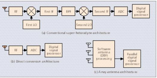
Figure 1. Various configurations for software-defined radio systems (receiver side).
