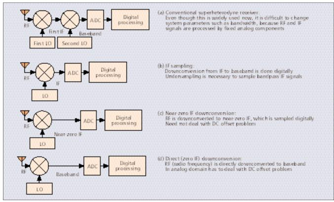
Figure 2. Types of down conversion in receiver.
