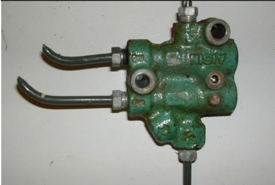
Up-left: the adjuster for the parking brake; right – the disk brake installed Below left: proportioning valve (not used); right – caliper with brake line and pads
