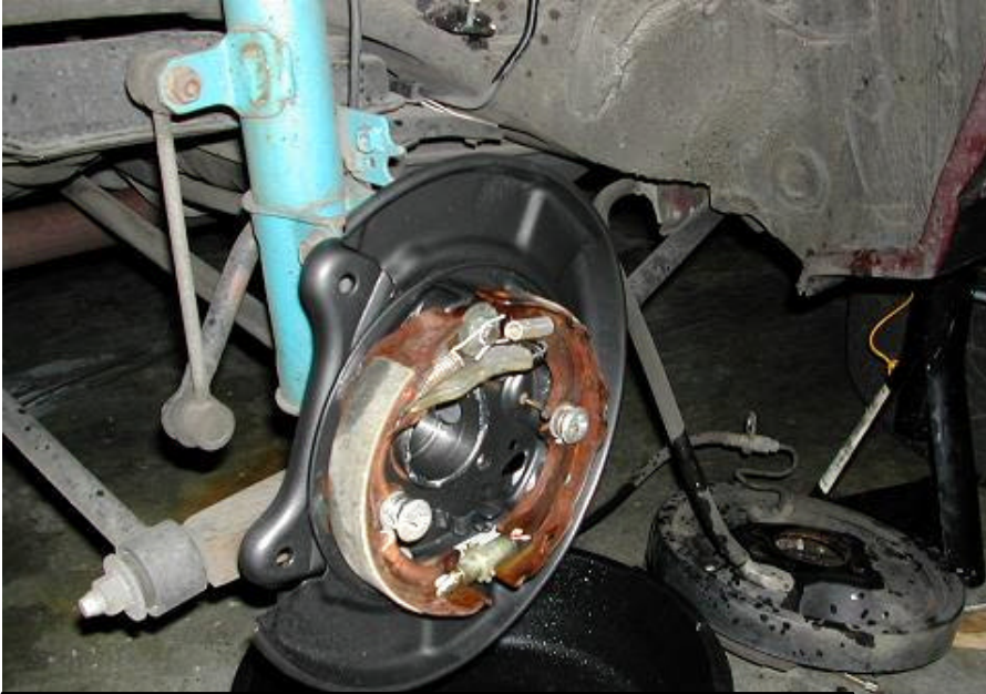
Up-left: disk brake backing plate installed (old brake still hanging by the parking brake cable); right – the hub off the car Below left: removing the spring plate from the brake
