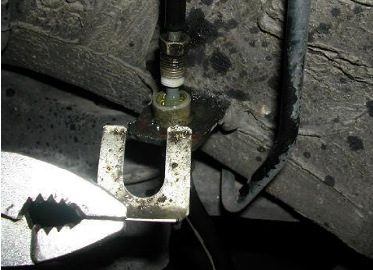
Up-left: disk brake backing plate installed (old brake still hanging by the parking brake cable); right – the hub off the car Below left: removing the spring plate from the brake
