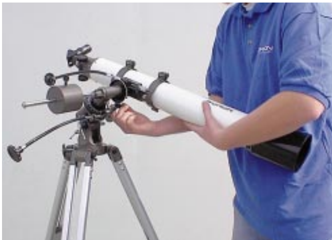
Figure 2c. Preparing the telescope to be balanced on the Dec. axis by first releasing the Dec. lock knob.
