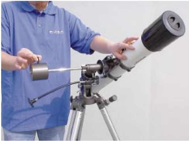
Figure 2a. Balancing the telescope with respect to the R.A. axis by sliding the counterweight along its shaft.
