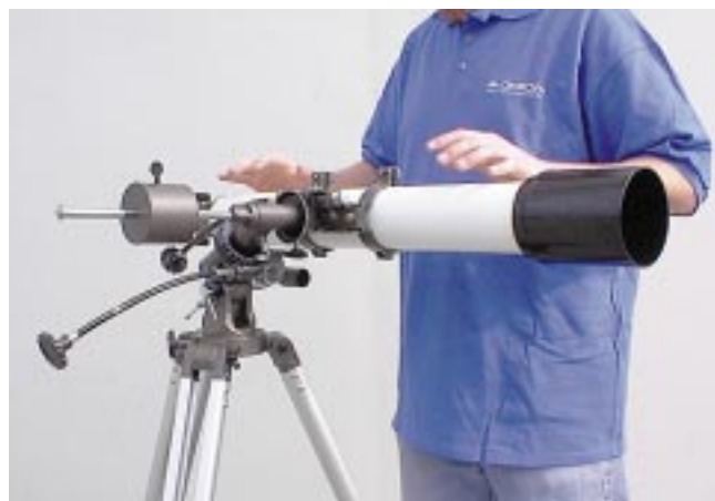
Figure 2e. Telescope is now balanced on the Dec. axis, i.e., it remains horizontal when hands are released.
