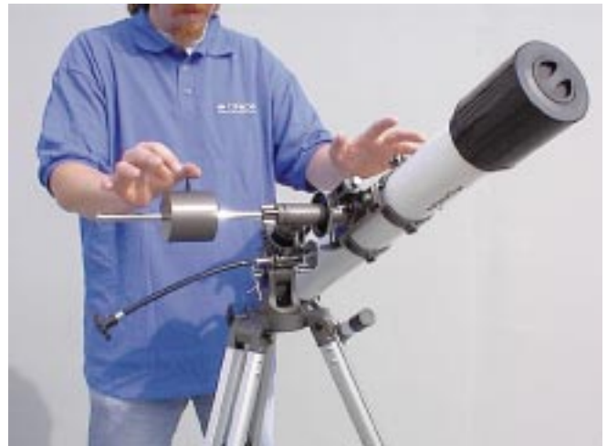
Figure 2b. Telescope is now balanced on the R.A. axis. That is, when hands are released, counterweight shaft remains horizontal.
