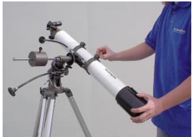
Figure 2d. Balancing the telescope with respect to the Dec. axis. As shown here, the telescope is out of balance (tilting).
