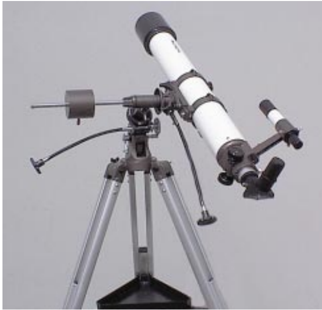
Figure 5a. Telescope pointing south. Note that in all these illustrations, the mount and tripod remain stationary; only the R.A. and Dec. axes are moved.
