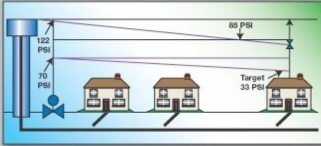
Figure 3. Pressure modulation in a basic hydraulic-based system.
