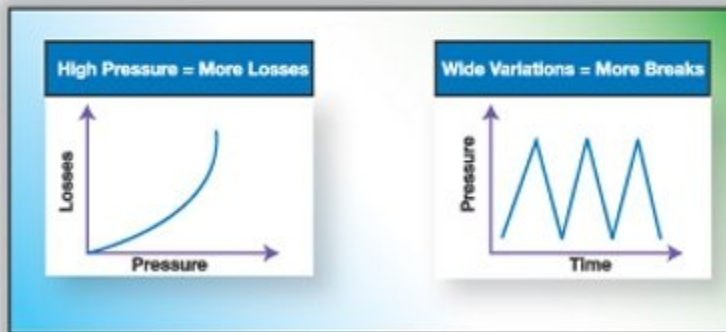
Figure 2. Excessively high pressures and wide variations in pressure equate to greater leakage losses.
