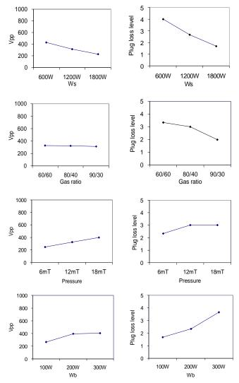
**Fig.2:** Individual etch parameter (Ws, gas ratio, pressure and Wb) effects on plasma potential and W plug loss.
