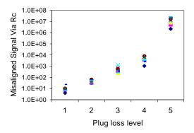
**Fig.3:** Electrical test result shows misaligned via resistance as a function of plug loss level.
