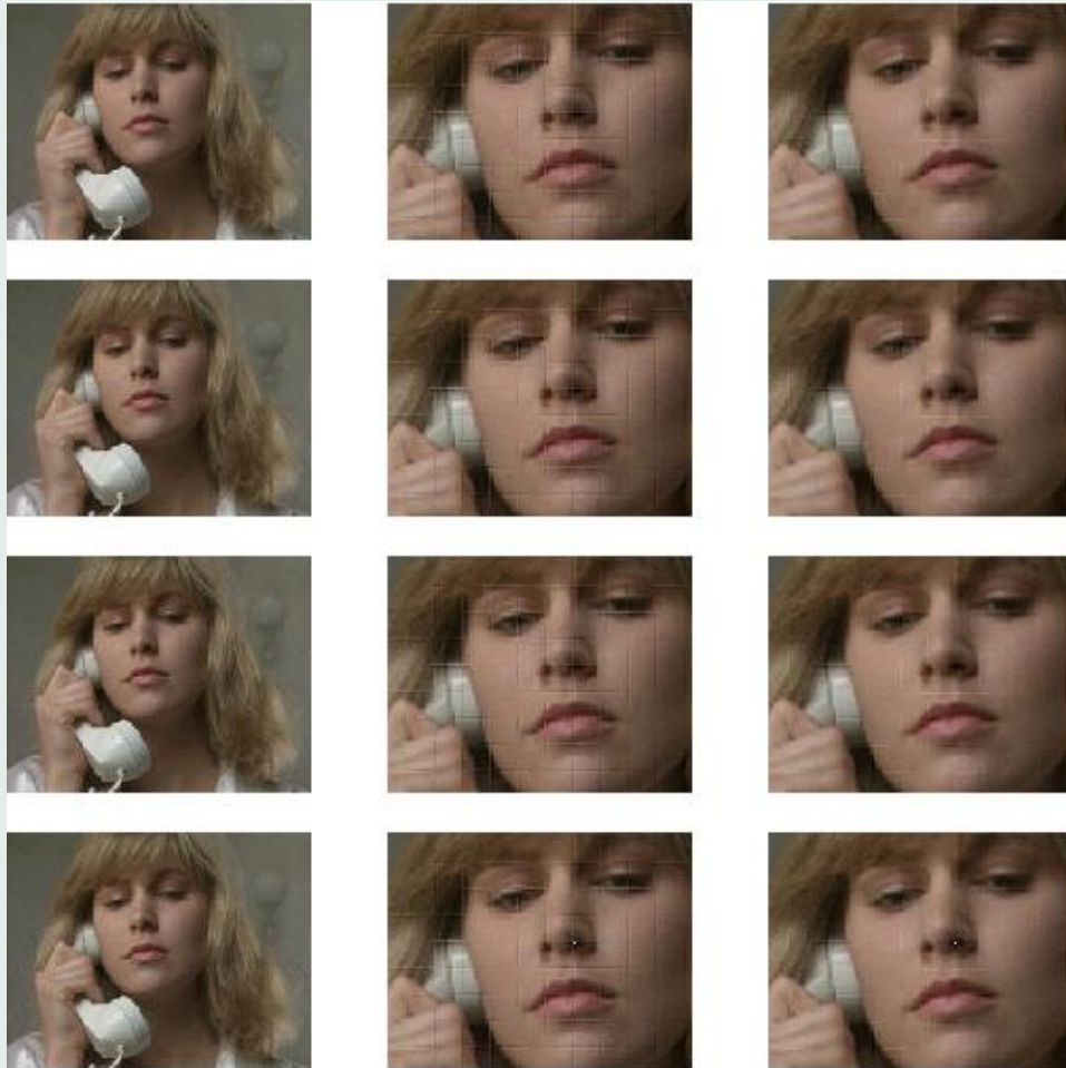
Suzie video clip. Left col:Original, Middle DCT, right DWT
