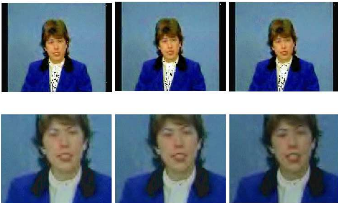
Figure 6.19: MRME based decompression and zooming. Top row shows decompressed Claire video after compressing at 11Kbps. Bottom row is zoomed version of the same compressed video clip
