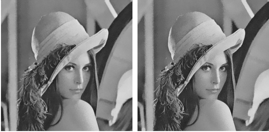
Figure 3: Successful attacked images of Lena. Left: pixel reallocation and median filtered, window size 8, threshold 15, PSNR 32.16. Right: pixel reallocation only, window size 8, threshold 20, PSNR 29.40
