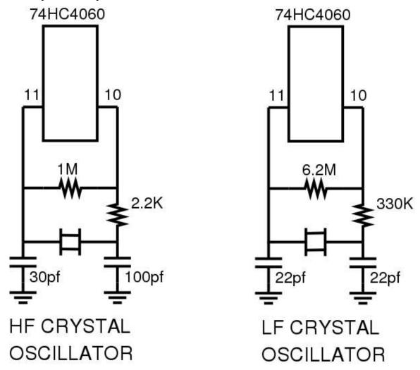
The circuit on the left came from the Fairchild data sheet on the 74HC4060 IC. Using these component values for my oscillator is where I got into trouble. While this circuit will work OK for HF crystals, the much smaller LF type watch crystals do not require, and cannot stand, such a high level of drive. With cheap tuning-gork type watch crystals this circuit will cause them to oscillate in strange off-frequency modes...just before they
