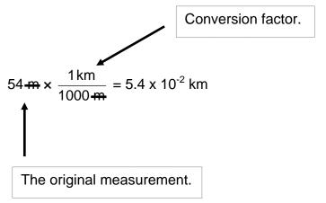
An important fact to remember is that you are not allowed to change the number of significant digits. These were determined at the time you made the measurement by the precision of your equipment. After the measurement is taken, the number of significant digits are etched in concrete!
