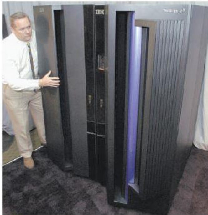
Figure 1-23 Mainframe computers can handle thousands of connected computers and process millions of instructions per second.
