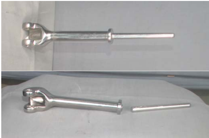
Fig.1. Prosthesis (a) Before failure, (b) After failure
