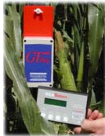
Measurements from soil sensors connected to this low cost data logger can be logged every 2 hours
