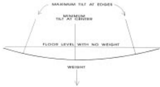
FLOOR, ROOF TILT FROM PERSON FIGURE 6.4
