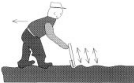
PUSHING DOWN AGGREGATE
