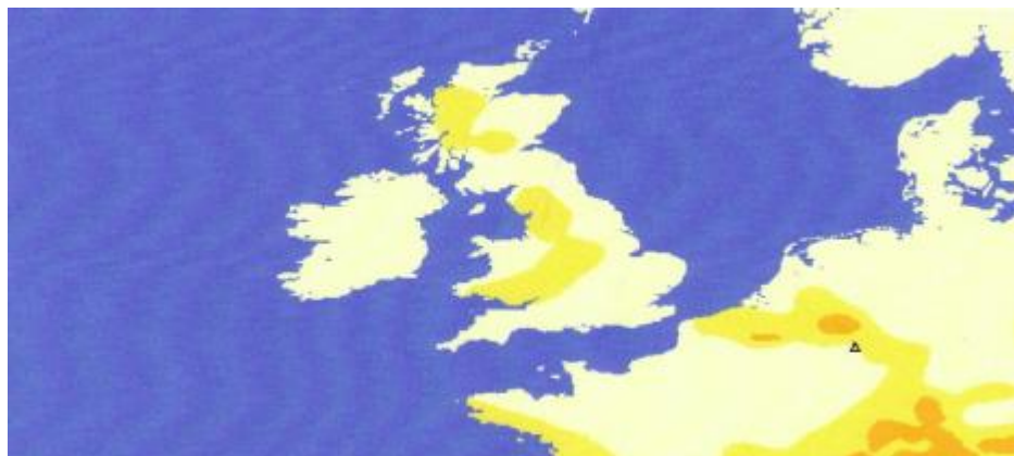
Figure 31: Regions of Raised Seismic Intensity, UK and Continent, The darker the yellow colour, the more seismically active the zone.
