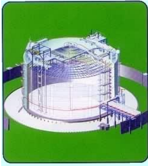
Figure 20 Design of typical Above-ground LNG Storage Tank.
