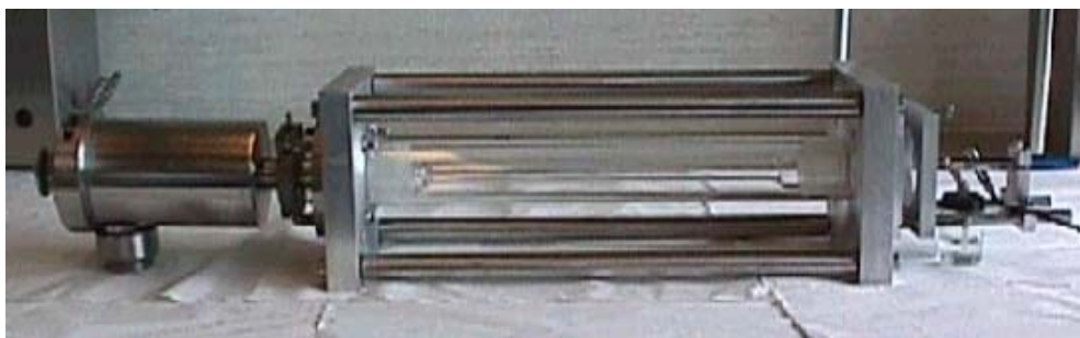
Figure 12: Airbrush system for generating particle standards (from left to right: Berner impactor, evaporation tube, airbrush)
