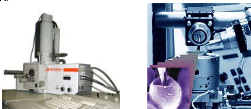
Figure 9: SEM-Raman instrument (left) and nanomanipulators (right) 52,53
