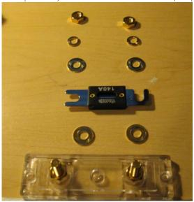
(From bottom to top - the ANL Fuse block base, flat washers, ANL fuse, flat washers, split lock washers, and hex nuts. These are actually stacked, in the picture, in order of assembly. The cabling has been omitted for clarity.)
