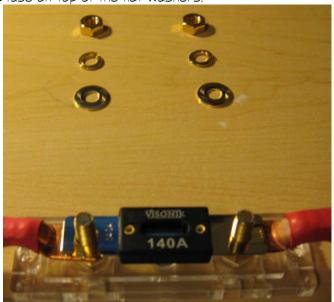
And now, the other pair of flat washers - the purpose of the flat washers, in case you're wondering, is twofold - they increase the contact area for electricity to pass through the terminals, and they also keep turning the nuts from deforming the contacts. The ANL fuse goes between the washers and the lugs under them so you don't have to wrestle with everything if/when you have to change the fuse. If the fuse goes between the washers, you won't hang up on any lugs - they're under the washers.
