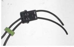
Insert the wiring "tails" up through the *bottom* of the fuse holder body. Which side is the bottom? Remember which side you took the seal out of in the first place? That's the bottom.
