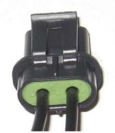
And reinstall the tan body-to-cap seal if you took it off before (you should have – it helps keep that seal from getting buggered up):
