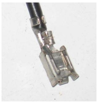
I decided to *not* reduce this for printing – so it's a full-size pic. Note what I described earlier – the "double fingers" get crimped over the bare wire, and the "single fingers" at the far end get crimped over the insulation proper – this helps with retention of the wire in the terminal.
