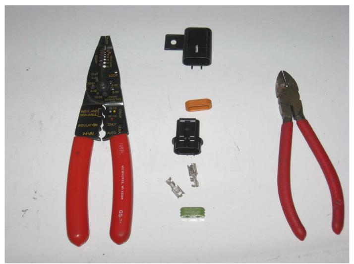
The above image shows you what you should have gotten in the kit (the centre "stack") and the tools you'll need to assemble your fuse holder (wire cutters on the right, stripper/crimpers on the left. Yes, most stripper/crimpers have wire cutters – but they've never worked well for me. Thus, the separate cutters.)
