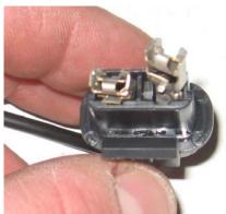
When you start to pull the terminals back into the house, you can see here how it should happen. There are locking tabs on the backside of the terminals, and they should go on the same side as the small grooves in the housing – those are there so you can release the locking tabs with a pick, if you need to. Gently press them in (you can use a flat surface to get them flush, then a small rod to get them the rest of the way) until they click – should look something like this:
