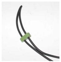
Insert the wiring through the green seal. It should be a slip-fit – that's how it's going to seal (the seals provided should work with 12-16AWG wire, which is about what you want for most circuit supply anyhow.) Leave plenty of "tail" past the seal – you'll need it while you finish putting it all together, although most of it will be coming back out.
