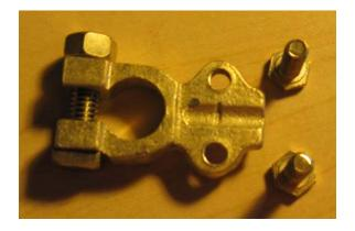
This is essentially a "universal repair" clamp with the strap removed (it was brass-plated steel anyhow.) I've never liked using a strap over a stripped wire on a battery, and I've never done it for long (just to get home, mainly.) You've probably bought a set of my battery cables, so you've got an idea how I do things.
