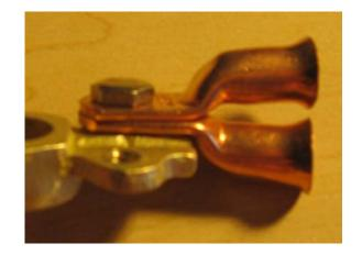
Here, you can clearly see that the lugs are "back-to-back," and that allows them to be properly secured with the shorter screw. You could put them "belly-to-belly," but that would require machining a spacer to keep the screw (and stack) tight. No, I don't have measurements – but I can probably tell you what you'd need, if you ask nicely and are patient.
