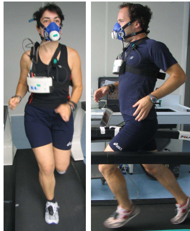
Figure 1: Obtaining heart rate and oxygen uptake data in a maximal oxygen uptake test (first and second authors).
