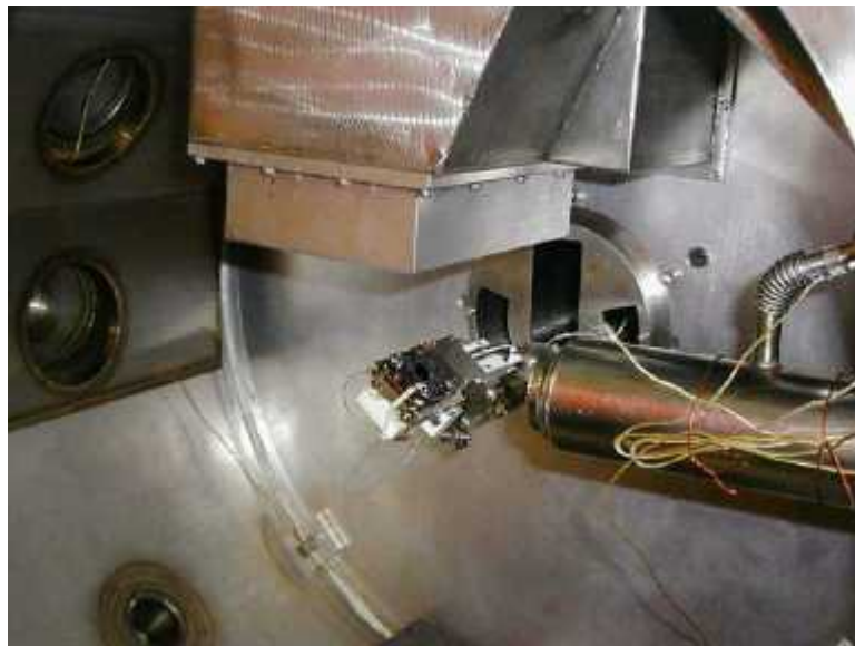
Figure 2.3 A very good view of the three elements: ioniser, the surface and the beam source unit.
