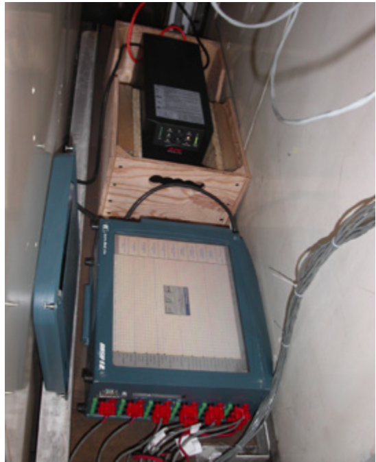
FIGURE 9. ASTRO-MED DASH-18 DIGITAL CHART RECORDER IN FOREGROUND AND UPS IN THE BACKGROUND.
