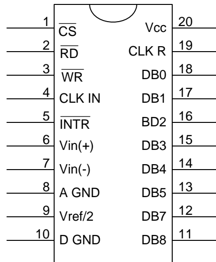
Figure 7. ADC0804 pin out
