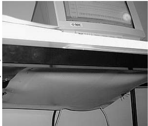
Figure 2.7 The foil installed under the table; only the polyethylene covering is visible.
