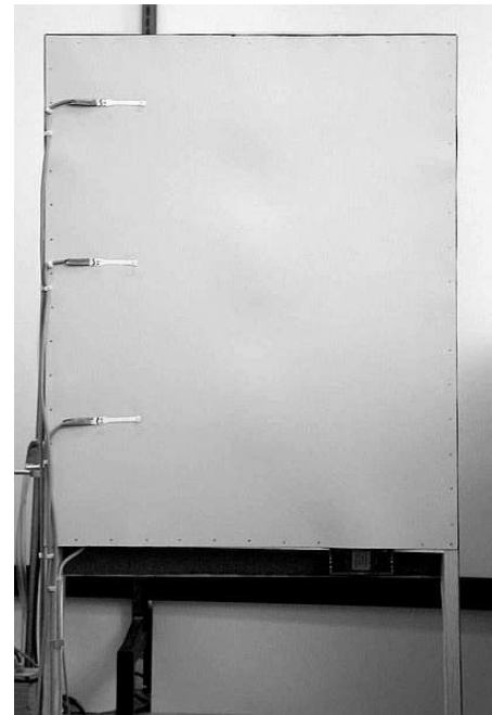
Figure 2.23 Surface temperature measurement with thermistors on the back panel of workstation 3.
